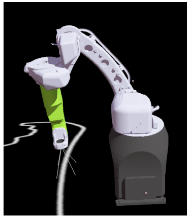
Fig. 5. Simulating the robot and the glue bead.
